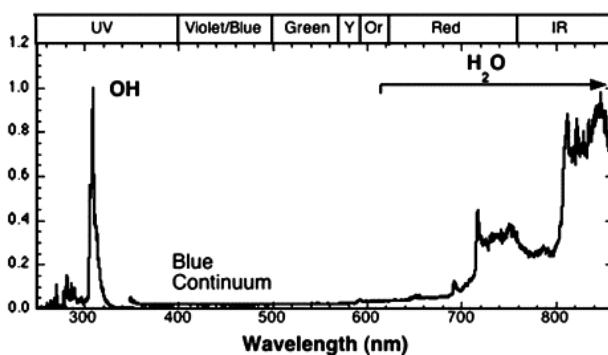
Figure 2: Spectrograph of an oxyhydrogen flame
