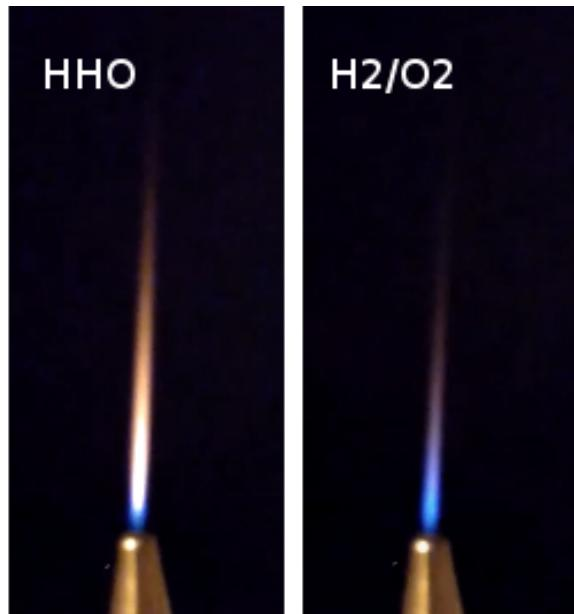
Figure 1: HHO flame vs. oxyhydrogen flame
